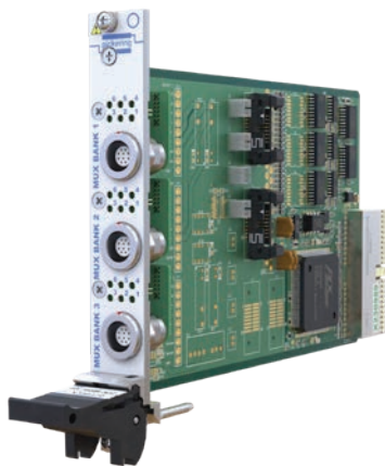
Single slot version controls 1, 2 or 3 remotely mounted multiplexers via interface cables
